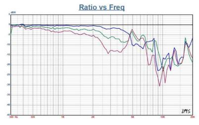
Figure 12: Dayton Audio DSA175 normalized on- and off axis frequency response (black solid =  $0^{\circ}$ , blue dot =  $15^{\circ}$ , green dash =  $30^{\circ}$ , purple dash/dot =  $45^{\circ}$ ).
