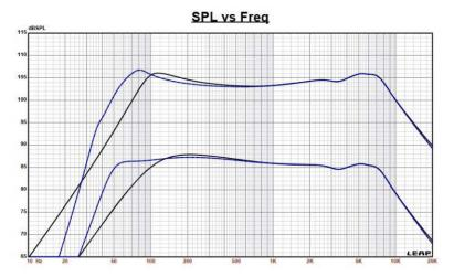
Figure 2: Dayton Audio DSA175 computer box simulations (black solid = sealed @ 2.83 V; blue dash = vented @ 2.83 V; black solid = sealed @ 40 V; blue dash = vented @ 40 V).
