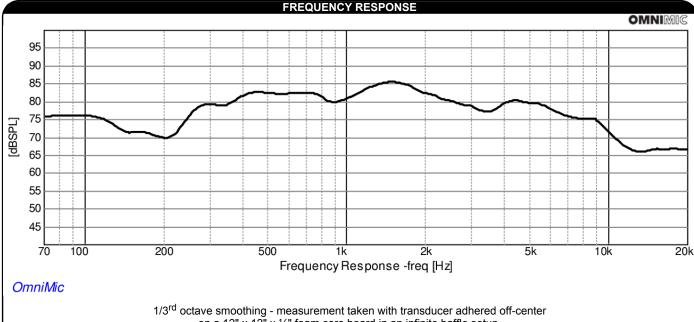
on a 12" x 12" x 1/2" foam core board in an infinite baffle setup.
