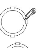
If the ceiling is made of drywall, simply cut the marked area with your utility knife or drywall saw. If the ceiling is made of plaster, you should use a saw with a higher tooth count to reduce the chance of breaking the plaster. Test fit the speaker in the hole, the speaker should fit loosely and the speaker frame should cover the edges of the hole. Repeat these steps for the other speaker.
