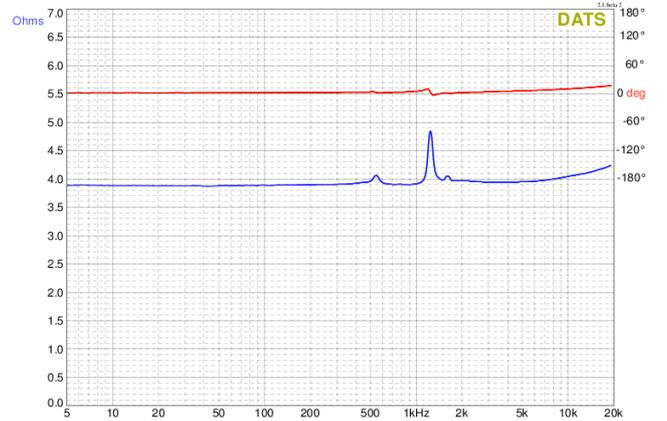
Measurement taken with transducer uncoupled facing upward.
